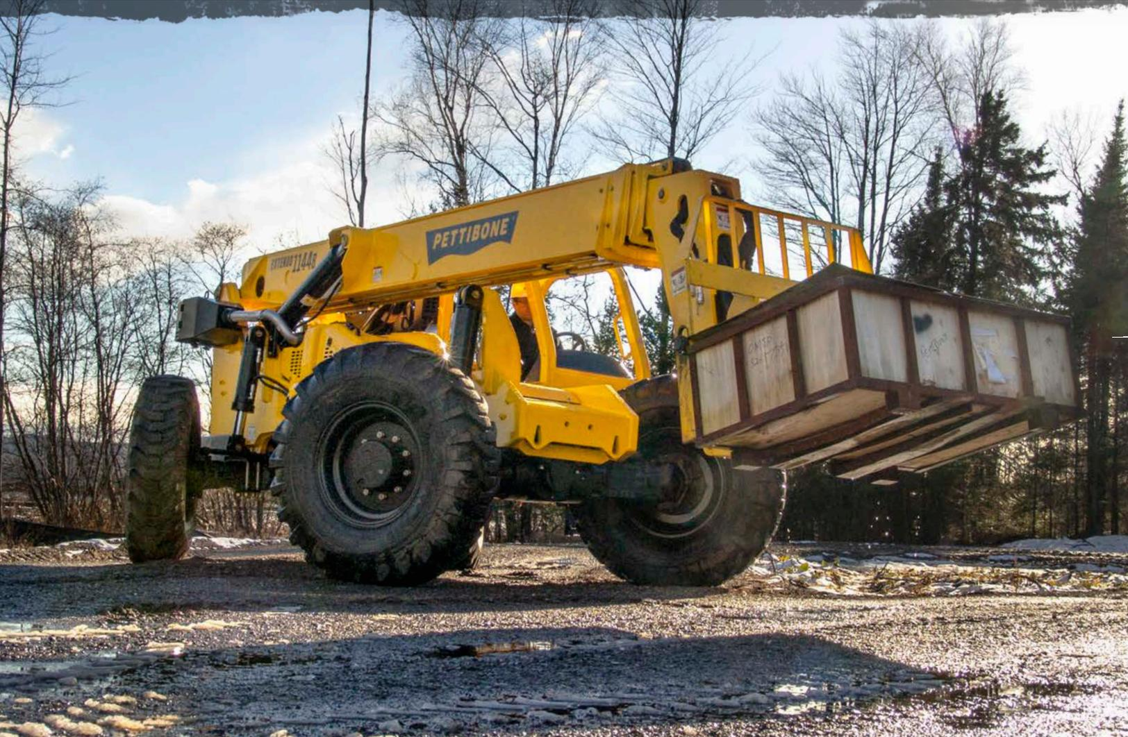
The Pettibone® Extendo™ 1144B telehandler offers exceptional material handling capacity and maneuverability for a variety of applications. Providing excellent visibility from the cab, the 1144B allows operators to work safely and efficiently. Responsive hydraulics let users move loads with confidence, while superior engineering and service features maximize machine uptime.
