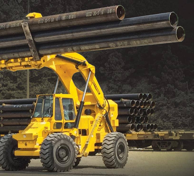
Rather than an articulating joint, the Cary-Lift has a solid steel frame that allows it to take full loads into sharp turns without affecting load capacity or stability.
