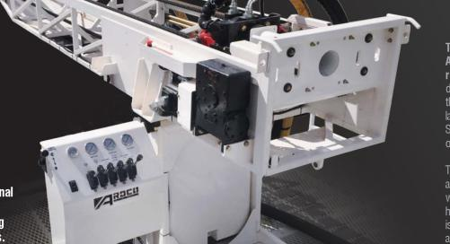
The first skid drill model is the SD350, ARDCO's skid mounted, vane-style water rotary drill rig. Powered by hydraulic pumps driven by auxiliary power or truck engine, this skid drill is ideal for seismic drilling on land up to 350 feet (107 meters) deep. The SD350 can be mounted on an ARDCO 4x4, on-road truck, or rubber tracked crawler.
