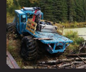
Allison six-speed automatic transmission, a Cummins 190 hp turbo-diesel engine and John Deere differentials that can be locked with the push of a button to boost traction under the most difficult conditions. It also features a 20,000-pound-capacity winch on the front end. made by Ramsey Industries. and a 3,500-pound-capacity picker crane, made by F.lli Ferrari Corp. S.p.A.
