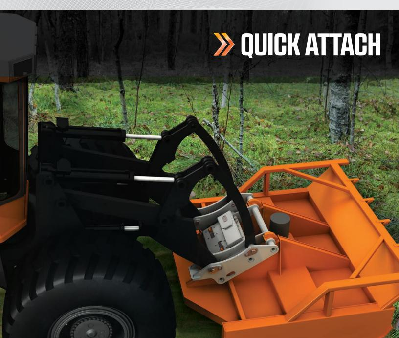
The Barko® Quick Attach gives users the flexibility to quickly and easily change between industrial tractor attachments for varying job requirements. With customizable specifications and the ability to deliver variable hydraulic flow and pressure, the Quick Attach can universally accommodate the requirements of any common attachment.
