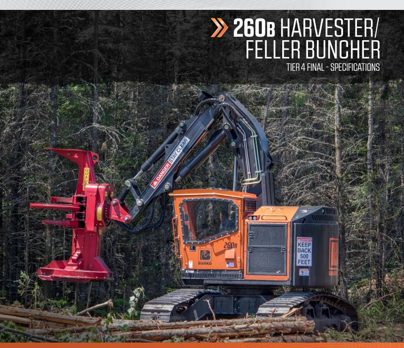
Equipped with a smooth, responsive IQAN® hydraulic control system, the Barko® 260B Track Harvester/Feller Buncher delivers an optimal combination of strength and efficiency. Purpose built with engineering input from forestry professionals, the Barko 260B offers exceptional drawbar pull (1.13:1 ratio) and intuitive maintenance features for superior reliability.
