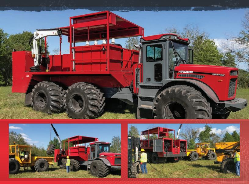
The ARDCO® AMT 600 Service and Lube Station includes a wide array of product delivery systems, including tanks for diesel, oil, coolant, grease and e-vac. Featuring a steel-constructed body platform with sheet metal roof structure, the station also includes ancillary equipment such as an air compressor, pressure washer, welder and crane.
