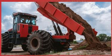
The 10-ton payload ARDCO® AMT 400 Dump Bed provides 8 yards of capacity, or up to 12.5 yards with added sideboards. The dump bed can also be easily removed as needed to transform the unit from an articulating dump truck to a multi-purpose vehicle for other jobsite tasks.
